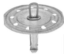
For base sheet, recovery board, and insulation attachment to lightweight insulating concrete, structural woodfiber, and poured gypsum. Formed from coated steel to prevent corrosion, the twin loc-nail easily penetrates decking and existing membranes.
