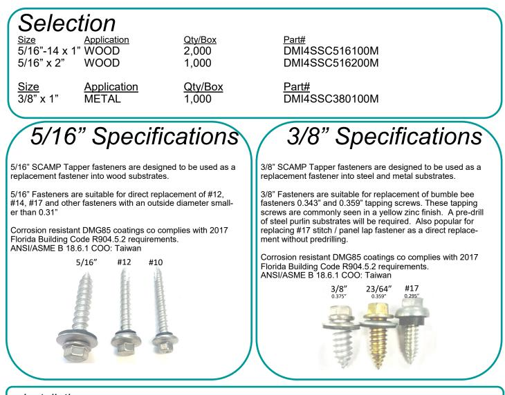
**Installation:** 3/8" Hex driver LSC drivers suggest. 0-2500 rpm electric screw gun with depth sensing nose piece or torque control device. Suggested drill speed into most substrates is1800 rpm. Do not overdrive or under drive, not suggested for use with impact driver installation tools. Approximated values are average ultimate values. Values may change with strength and condition of substrate wood or steel.
