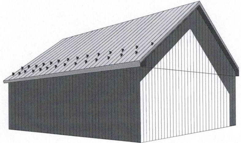
Snow Trax spacing shown is for example purposes only. The design for each individual roof is based on several factors and building geometry.
