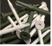
XLP WTM SD3, SQ2, Metal 22ga up to 6 ga Available Sizes Oty/Box Part# 2,500 DMIXLP101780S3 #10-16 x 1-7/8' Popular for plywood & OSB decking or 1"x4" dimensional lumber to metal deck or purlins.
