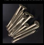
The XLP CON features #2 square drive for stability, torque relief thread and DMG95 1500 hour exterior coating available in white or bronze. The XLP CON is popular for window installation and wood to concrete attachment.
