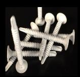
The XLP SD features a self drilling point designed to drill and tap into steel up to 6 gauge thickness. Popular for securing plywood to metal decking or framing. Also popular for window and door installation.
