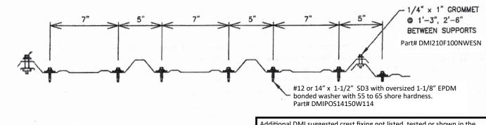
Additional DMI suggested crest fixing not listed, tested or shown in the Texas Department of Insurance T.D.I. installation guide.
