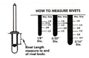
\* Body Length is approximate (& doesn't include countersunk or large flange.)
